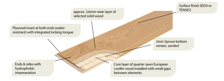
**Product description** Multilayer parquet with a 3-layer construction for glueless installation
